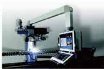
Stellite PTA Welding Machine for Bimetallic Screw
